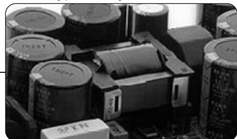
Switching power + Digital module ( 600W )
